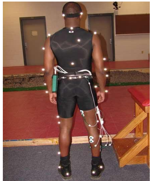
Figure 2. Markers and EMG Electrodes on the Rear Side of a Subject.
